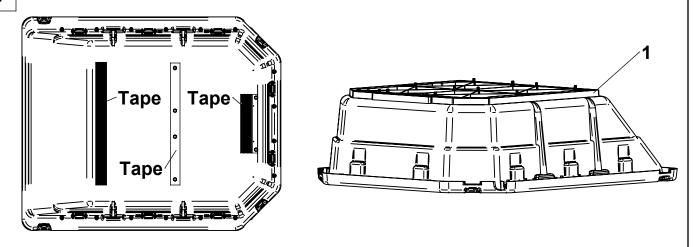
TIP: Bolt heads can be secured with tape to aid in asembly.
