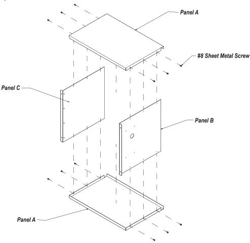
4. Position the assembled filter box on rear of furnace, supporting it firmly up to electrical enclosure, covering the rear distribution blower.
