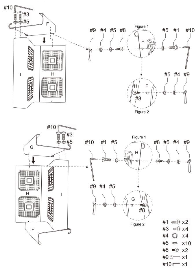
Step 6. Using at least two people, carefully lift assembled unit (parts F, G, H & I) and place inside assembled unit (parts A, B, C & D).
