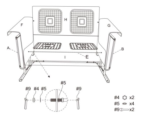
Step 8. Attach connecting wire (part E) to arms (parts F & G) using metal washers (part #5), self-locking nuts (part #4) and wrench (part #9).
