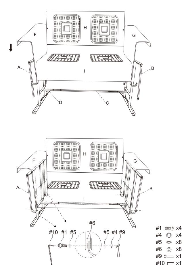
Step 7. Attach connecting wire (part E) to arms (parts F & G) using metal washers (part #5), self-locking nuts (part #4) and wrench (part #9).
