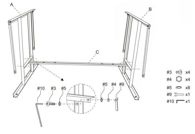
Step 3. Attach supports (part D) to legs (parts A & B) and leg support (part C) using short bolts (part #3), metal washers (part #5), self-locking nuts (part #4), wrench (part #9) and allen wrench (part #10).
