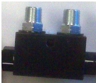
Check valve with BSPP-NPT adapters installed
