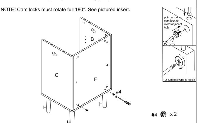
Step 7. Attach top panel (part A) to left side panel (part B), right side panel (part C) and back panel (part F) using wood dowels (part #5), cam locks (part #4) and phillips head screwdriver.
