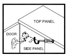
Loosen the screw indicated a little, adjust the hinge to right position (see step 2a & 2b), then tighten the screw.
