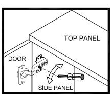
Loosen or tighten the screw indicated a little to adjust the gap between doors panels (see step 3a & step 3b)
