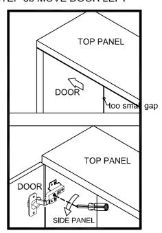
Turn the screw counterclockwise a little as shown to make the gap big.
