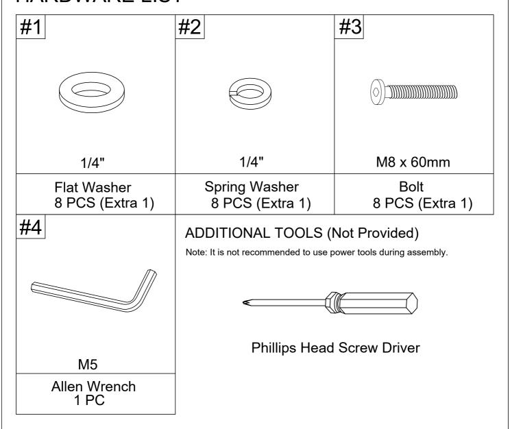
Step 1. Before assembly remove four wood connectors (See Figure 1) and two corner connectors (See Figure 2) using phillips head screwdriver. Carefully place table top (part A) on a soft flat surface, such as carpet. Attach legs (part C) to table top (part A) using spring washers (part #2), flat washers (part #1), bolts (part #3) and allen wrench (part #4).
