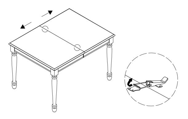
Step 3. Place table leaf (part B) in position and push table top (part A) from both ends to close.
