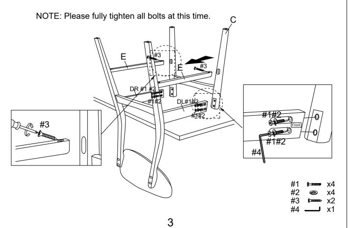
Step 3 . Attach seat (part B) to side rails (parts DL & DR) using screws (part #3) and phillips head screwdriver.
