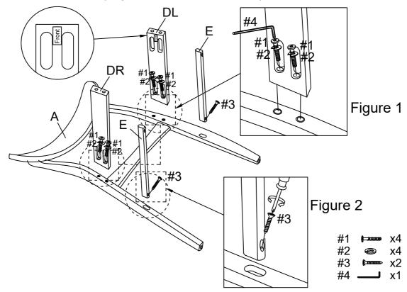
Step 2 . Attach front leg (part C) to side rails (parts DL & DR) and stretchers (part E) using bolts (part #1), spring washers (part #2), screws (part #3), allen wrench (part #4) and phillips head screwdriver.
