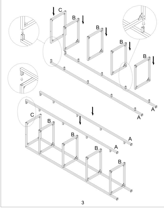
Step 2. Secure top shelf frame (part C) and shelf frames (part B) to the legs (part A) using bolts (part #1) and allen wrench (part #2). Bolts (part #1) will be inserted from the opposite direction for top shelf frame (part C) only.
