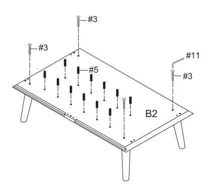
Step 4. Attach bottom partition panels (part G2) to bottom panel (part B2) and bottom shelf (part F2) using small wood dowels (part #5).
