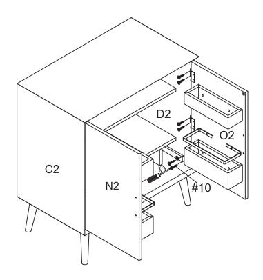
Step 12. Attach handles (part #9) to left door panel (part N2) and right door panel (part O2) using round head bolts (part #8) and phillips head screwdriver.
