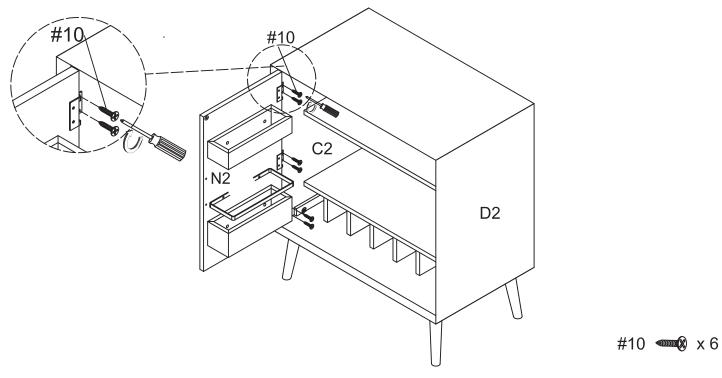
Step 11. Attach right door panel (part O2) to right side panel (part D2) using hinges (pre-installed), large screws (part #10) and phillips head screwdriver.
