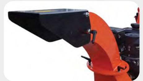
Rotational chip chute pickup truck bed height.
