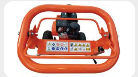
Large multi position adjustable Bow Handle. CE approved safety shut off.
