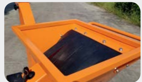
Large Feed Chute
