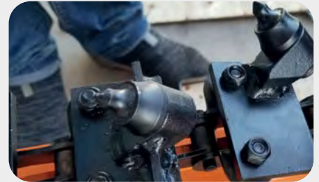
Tri-Cut High Carbide Teeth
