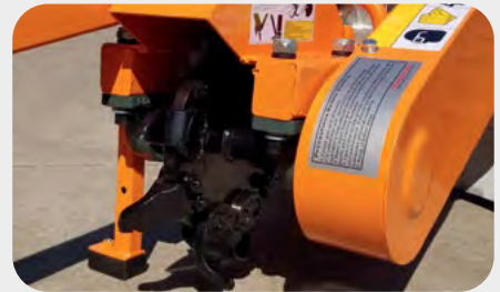
9 Carbide Cutting Head - Direct Drive
