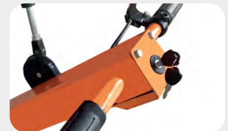
Lock out safety keys - Locking Throttle
