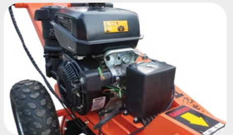
Dual direct V-Belt, high speed 3600 rpm drive.
