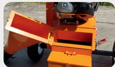
Extended Axle / Dual Swing Chutes / Tool Box
