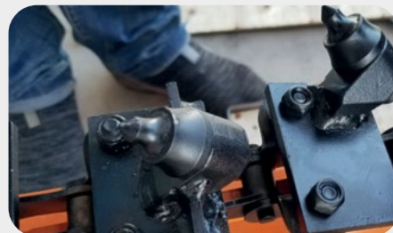
Tri-Cut High Carbide Teeth
