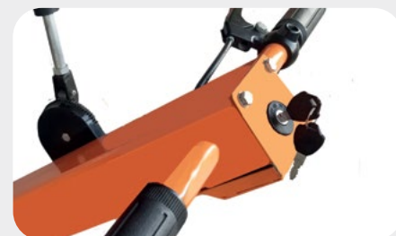
Lock out safety keys - Locking Throttle
