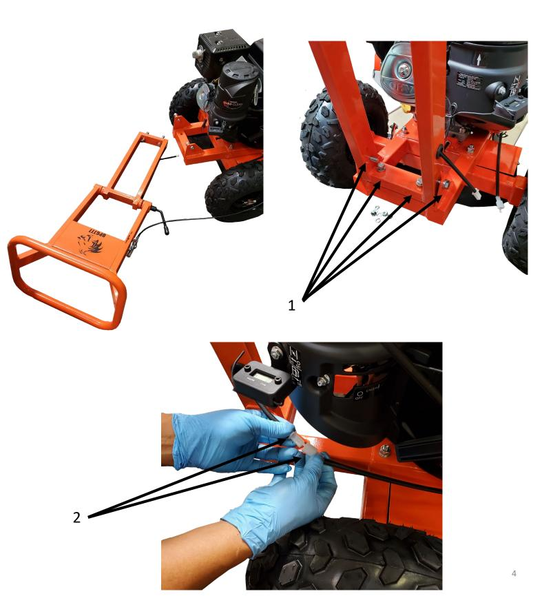
1. SECURE THE THROTTLE CABLE WITH THE LOOP WIRE CLAMP PROVIDED ON THE CHASSIS.
