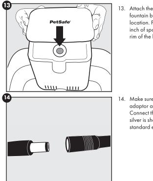
13. Attach the lid to the tower. Pick up the pet fountain by the bowl and place it in a desired location. Pour water into the bowl, leaving 1/2 inch of space between the water level and the rim of the bowl.
