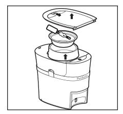
We recommend you wash and rinse the bowl, bowl holder, food hopper, lid and conveyor. Once parts are dry, ensure a conveyor belt lip is aligned with the arrows on the side. Replace the conveyor and food hopper.
