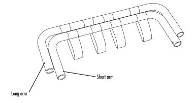
The longer arm should connect to the outter base tube. The shorter arm should connect to the inner base tube.
