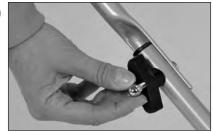
Cap the exposed bolt with an acorn nut (T13) and tighten with your 7/16" wrench until snug. Do not over tighten.
