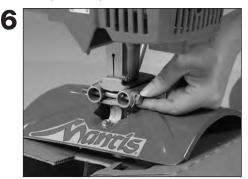
Slide the second 3-inch bolt (T11) through the second set of holes in the short legs. Add a lock nut (T14) and tighten finger tight until you've completed assembly.
