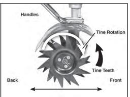
For cultivating, reverse the tines so that the points of the tines face backward - toward the operator. Now the long flat part of the tine's blade will contact the ground first.
