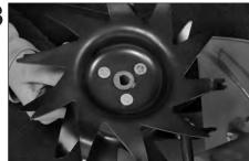
• You will notice that one side of the Tine has a circular hole while the other has a "D" shaped hole.
