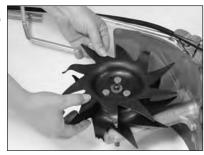
When the axle protrudes from the other side it will line up perfectly with the "D" shaped hole.
