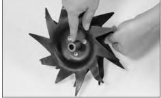
Attach the Tine so that the circular hole slides onto the axle first. 5
