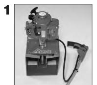
For ease of assembly and stability it is important that you keep the engine assembly in its cardboard cradle. 2
