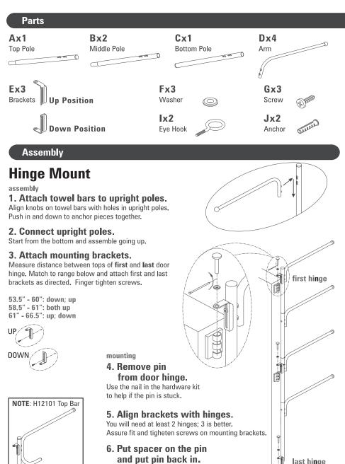
Hinge pin should pass through the plastic spacer,
