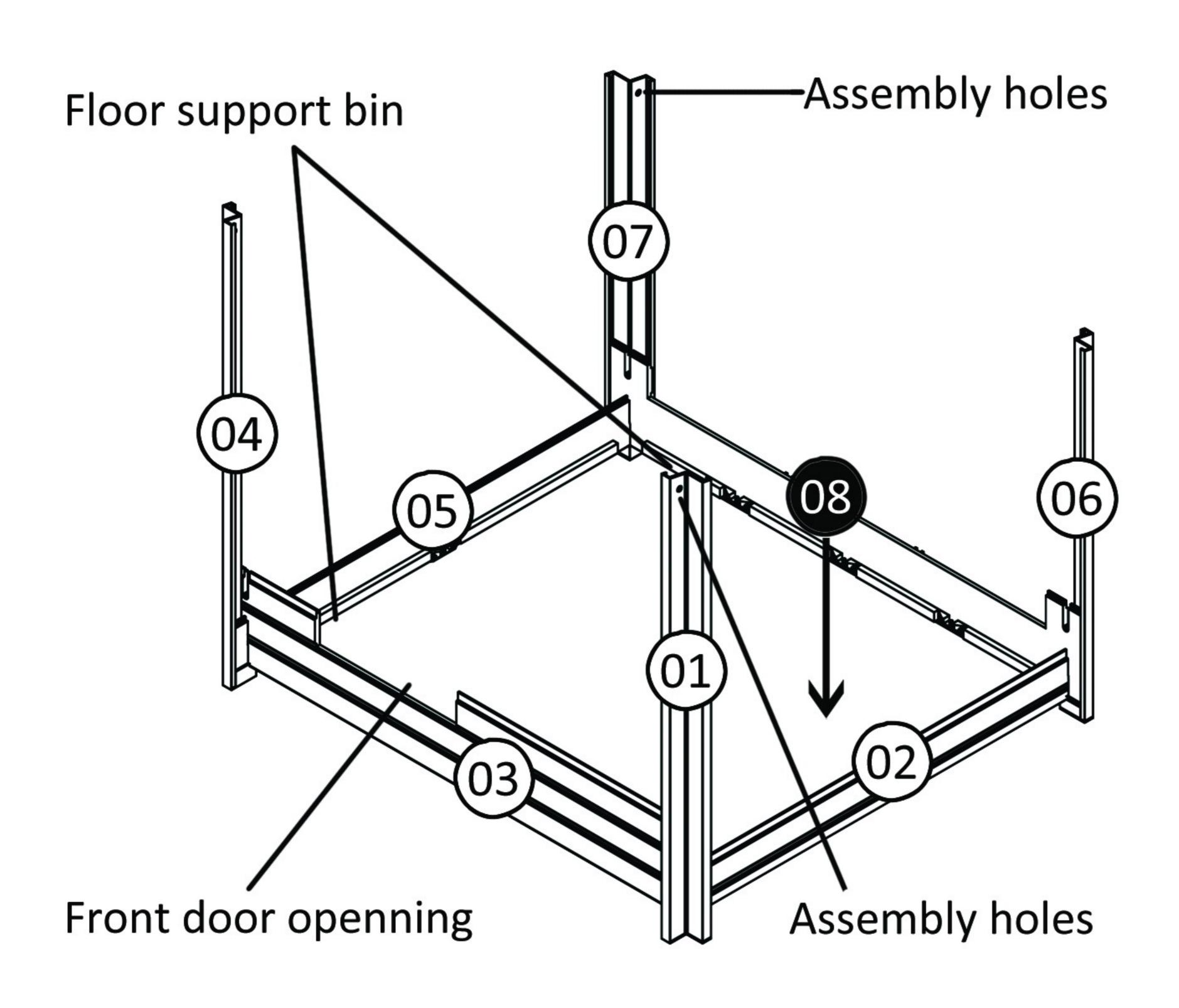
So far you have setup the wall base panels, (02), (03), (05) & (08); and the 4 column posts. Step back and stand facing the front door open. Do a quick check:
