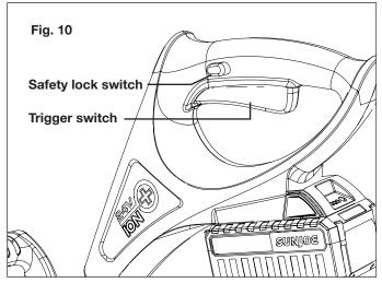
To stop the cordless snow shovel, release the trigger switch.
