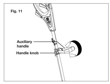
**3.** Fix the handle by tightening the handle knob. Insert the battery and resume working.
