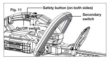
To turn the tool OFF, move the hedge trimmer away from cutting area, and release one of the switches (Fig. 11).
