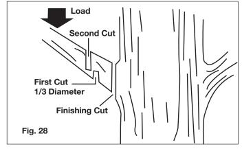
Now make your finishing cut from the topside of the branch smoothly and neatly against the main member so the bark will grow back to seal the wound.  Release the ON/OFF switch as soon as the cut is completed. Failure to follow proper cutting procedures will result in the bar and chain binding and becoming pinched or trapped in the limb.
