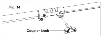
**3.** Follow the same instruction to fit the pole saw head assembly into the extension pole.
