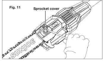
**NOTE:** If the chain is too tight, it will not rotate. Loosen the end cover nut slightly and turn the chain tensioner 1/4 turn counterclockwise. Lift the tip of the guide bar up and retighten the end cover nut. Ensure that the chain can be rotated by hand without binding.
