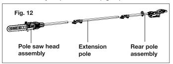
1. Align and insert the extension pole into the coupler on the rear pole assembly. Push hard until it is fully inserted into position (Fig. 13).
