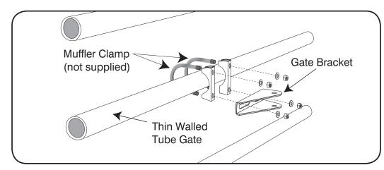
Muffler Clamp for Gate Bracket
