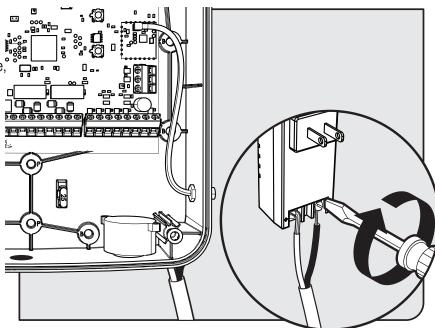
**MM372 Installation -** For dual arm installation, drill through one of the **Alternate Access** slots to install the Transformer or Solar power wires.
