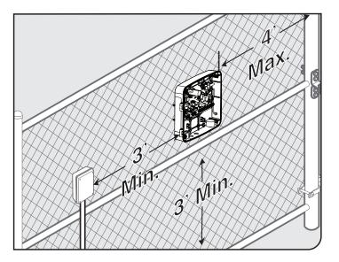
Identify a suitable mounting location for your control box at least 3 ft. from the ground and no more than 4 ft. from the primary operator.
