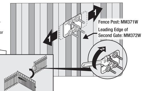
**Note:** For MM372W installations, the closed position stop plate should be installed on the leading edge of the PRIMARY gate leaf, and adjusted to close against the leading edge of the SECONDARY gate leaf.
