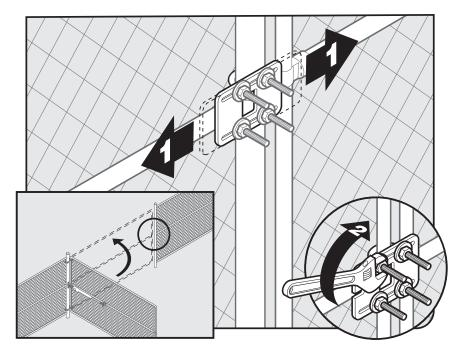
**Note:** For MM372W installations, the closed position stop plate should be installed on the leading edge of the PRIMARY gate leaf, and adjusted to close against the leading edge of the SECONDARY gate leaf.
