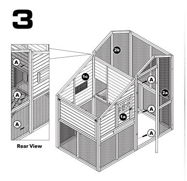
3. Connect Foraging Area Panels (2a, 2b) to Roosting Area Panels (1a,1c) with Screws (A).
