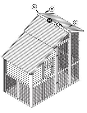
6. Attach Roof Cap (10) with Screws (C).
