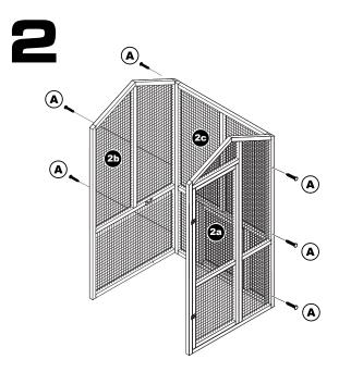
2. Connect Foraging Area Panels (2a, 2b, 2c) with Screws (A).
