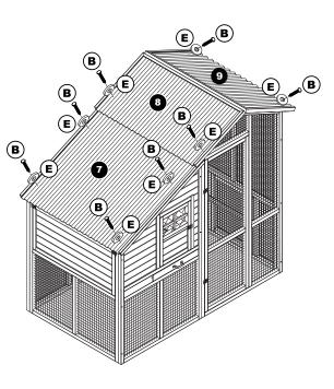
Attach Lower Left Roof Panel (7) with Screws (B) and Plastic Washers (E). Attach Upper Left and Right Roof Panels (8 & 9) with Screws (B) and Plastic Washers (E).
