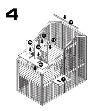
4. Insert Nesting Box Floor **(6a)** and Dividers **(6b)** into Roosting Area of coop.
