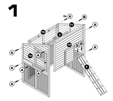
1. Connect Roosting Area Panels (1a, 1b, 1c, 1d) with Screws (A).
