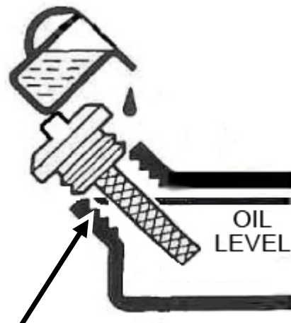
Figure 2 - Add Oil To TOP Of Threads
