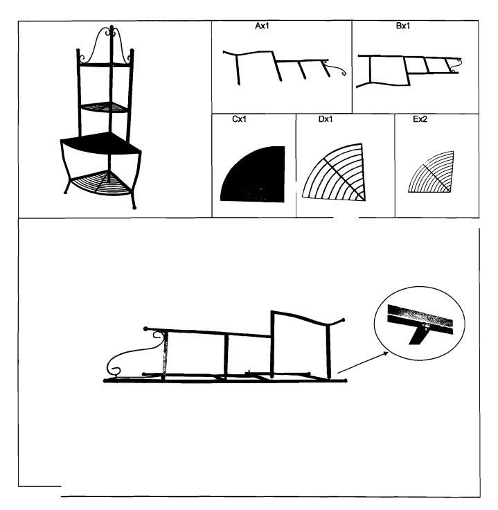
NOTE: PERIODICALLY CHECK AND TIGHTER BOLTED CONNECTIONS.
