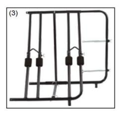
**Step 4**. Connect the left and right sections. A. To connect the back U-Frame sections, fit one Spacer Bar (F) between the top bars and one Spacer Bar between the bottom bars. Secure with two Clip Pins (H) per bar.
