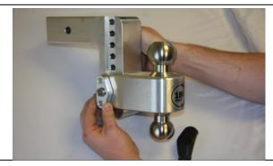
**STEP 4:** Pull on the <u>Keylock Assembly(WS03)</u> to ensure that it has been engaged. Do not operate without making sure <u>Keylock Assembly</u> is securely locked in place.
