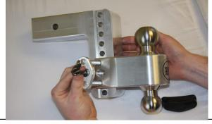
**STEP 3:** Insert the <u>Keylock Assembly (WS03)</u> into the <u>180 Slider</u> when you have achieved the desired position along the <u>Drawbar</u> and lock in place by turning the key.
