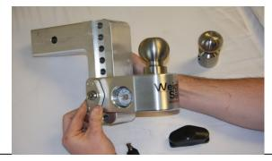
**STEP 4:** Pull on the <u>Keylock Assembly (WS03)</u> to ensure that it has been engaged. Do not operate without making sure Keylock Assembly is securely locked in place.
