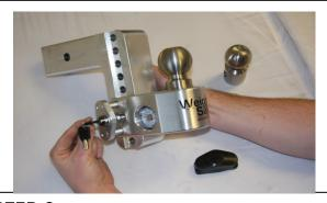
**STEP 3:** Insert the <u>Keylock Assembly (WS03)</u> into the <u>Weigh Safe Slider</u> when you have achieved the desired position along the <u>Drawbar</u> and lock in place by turning
