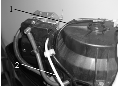
1. Start-in-gear protection cable 2. Choke cable
