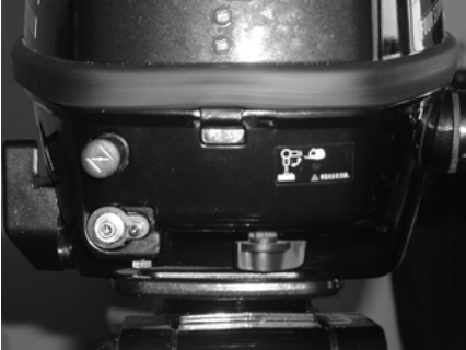
Built in fuel tank
