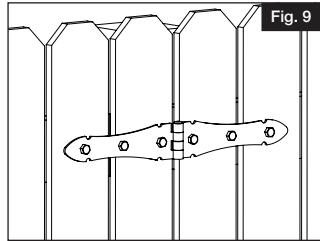
**NOTE:** Standard 8" Double Strap Hinges are NOT self-closing. If self-closing hinges are needed, a separate purchase of a Boerboel Gate Spring is required.
