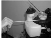
12. Give a strong pull straight out to crank and start the engine. Repeat it necessary.
