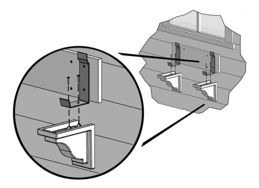
Secure each decorative corbel to the bottom of the wall mount brackets using two 3/4 inch screws. The decorative corbels are sold in pairs so we recommend installing them on the outside brackets. The molded corbels are only decorative so there is no need to over tighten the screws.
