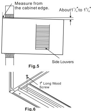
Refer to Step 5 of Window Mounting for assembly of support brackets. A wooden strip nailed to the outside wall should be used in conjunction with sill support angle brackets.
