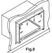
6. Install chassis into cabinet by following all steps in Step 8 of Window Mounting.
