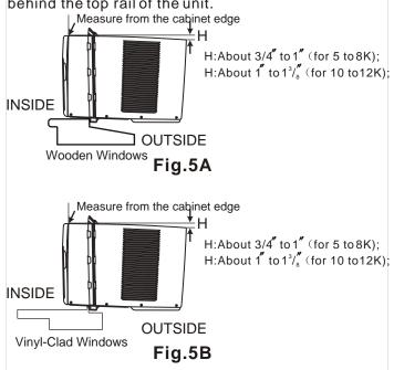
**NOTE:** Check that air conditioner is tilted back about H (Fig.5A and Fig.5B)(tilted about 3° to 4° downward to the outside).
