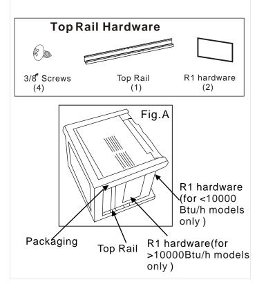
C: Align the hole in the top rail with those in the top of the unit as shown in Fig.B
