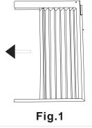
A.Place unit on floor, a bench or a table. Hold the Accordion Panel in one hand and gently pull back the center to free the open end. See Fig.1
