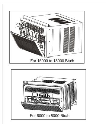
The air filter should be checked at least once a month to see if cleaning is necessary. Trapped particles in the filter can build up and cause an accumulation of frost on the cooling coils.
