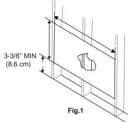
Carefully measure and cut an opening with the following dimensions depending on your model. See Fig.1 and Fig.2. WIDTH" X"= inside model width plus twice the
