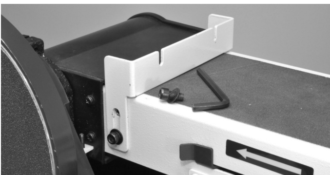
Figure 2 - Install small fence.
