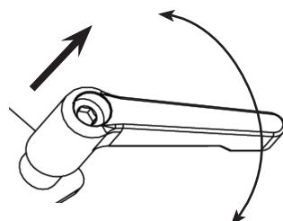
Your seeder comes with 2 adjustable handles for quick and easy adjustments on the Row Marker blade and the plow
