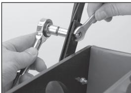
Using a 10 mm wrench to hold nut and a 10 mm wrench to secure bolt, tighten all 4 bolts to secure handlebar to hopper/wheel assembly.
