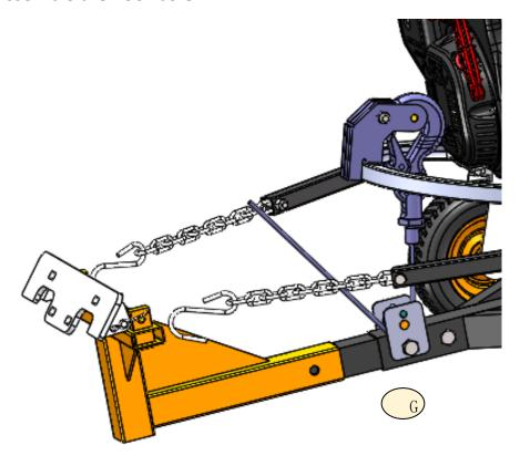
6. As H and I, put the chain on the UTV steel frame, then adjust the square tube and tighten the chain.
