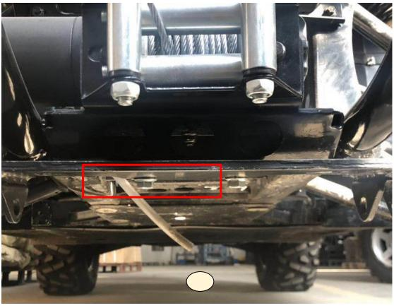
3, As D and E, assemble the connection bracket welded parts on the UTV, fixed by F.
