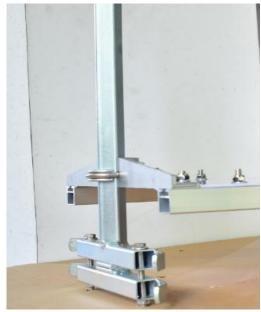
With the end post assembly attached to the frame bracket and long rails, adjust to desired cutting thickness (minimum 3 inches) and tighten nuts around U-Bolt.
