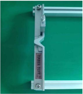
7. Attach chain guard assembly to the frame bracket (#6) using U-Bolt (#9)m U-Bolt Adaptor/Clamp (#10), washers (#11), and long hex nuts (#2).
