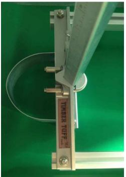
With the guard assembly attached to the frame bracket and long rails, adjust to desired cutting thickness and tighten nuts around U-Bolt.
