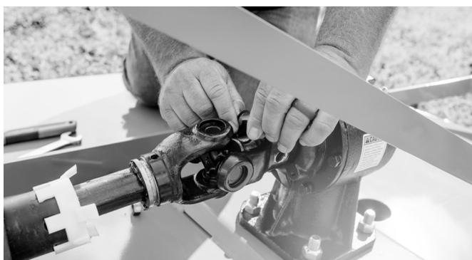
23. Align the shear bolt holes, install, and tighten PTO shaft shear bolt.
