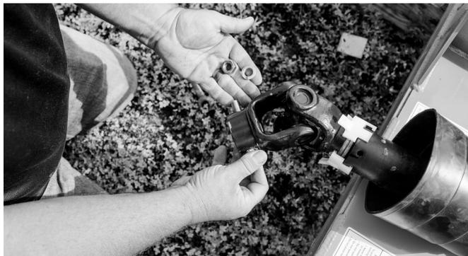
21. Slide the PTO shaft onto the gearbox shaft.
