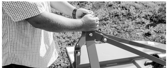
14. Go back and tighten the CAT I pins, on both sides, using a 1-5/16" wrench/socket.
