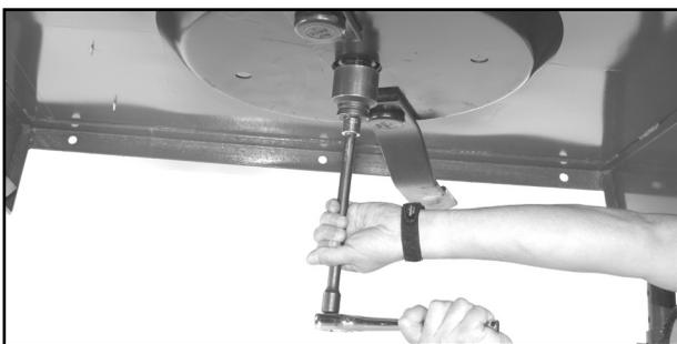
7. To reinstall blade pan, reverse the above steps. Be sure to tighten the castle nut and replace the cotter pin.
