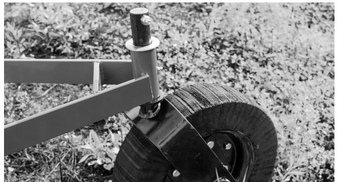
6. Using 1-5/16" wrench/socket, remove the CAT I pins from the shipping boots.
