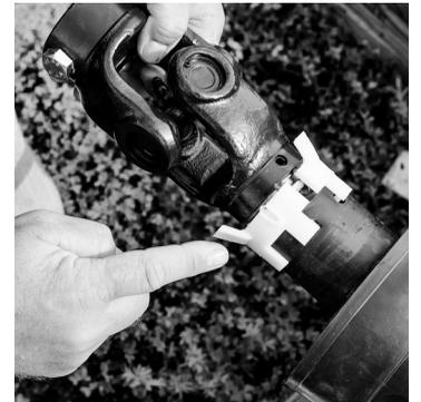
4. If needed, separate white tab collar and slide shield tube back.
