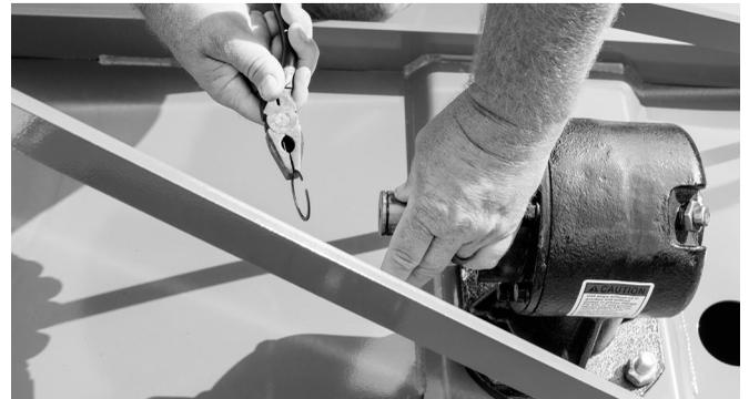
19. Slide the PTO shield back by using a screwdriver to apply pressure and release the locking collar. (There will be 3 tabs on the locking collar) Once the locking collar is released, slide the PTO shield back.
