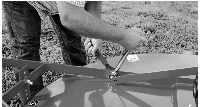
12. Place the backstrap brace on the bolt, as pictured, using the locknut. Hand tighten. Repeat for other side.
