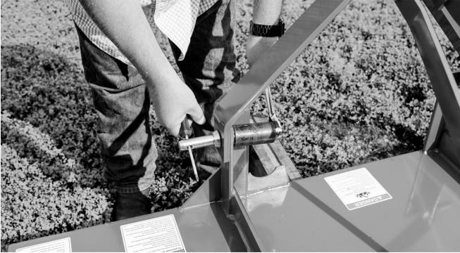
15. Tighten the nuts on the backstraps.
