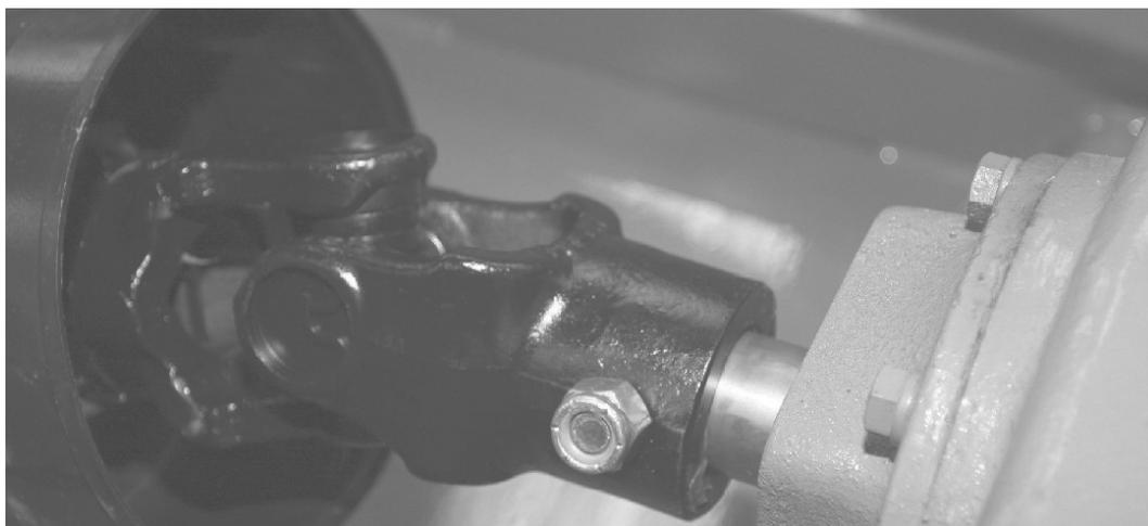
**NOTE:** Driveline shield pulled back for illustration purposes. Cutter drive components are protected from shock loads by a shear bolt.
