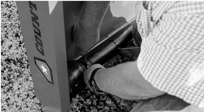
2. Remove 3/8" - 16 x 2" bolt and nut from the tailwheel holder on the shipping boot, using a 9/16" wrench.
