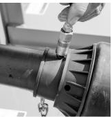
3. Re-install the PTO shield by sliding the shield over the universal joint making sure the shield locks in place.
