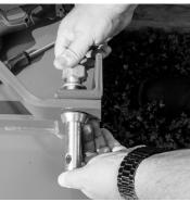
9. Remove the two zip ties from the tailwheel assembly and back braces.
