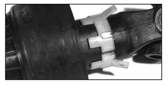
4. Slide collar shield into place until locked.
