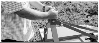
14. Go back and tighten the CAT I pins, on both sides, using a 1-5/16" wrench/socket.
