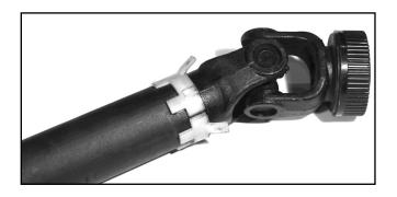
2. Slide driveline shield tube over white tab collar. Align slots/holes with holes in tube.
