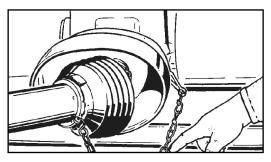
6. The PTO drive shaft must not be suspended from the chains!
