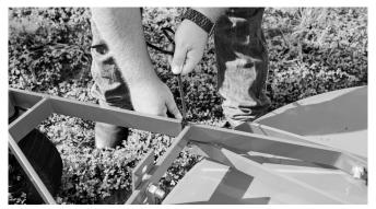
10. Raise the lift arms in the upright position, using the bottom pivot point.
