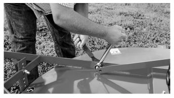
12. Place the backstrap brace on the bolt, as pictured, using the locknut. Hand tighten. Repeat for other side.
