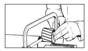
4. Round off all sharp edges and remove burrs. Grease sliding profiles. No other changes may be made to PTO drive shaft and guard.
