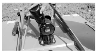
7. Replace and tighten both plugs on the gearbox.
