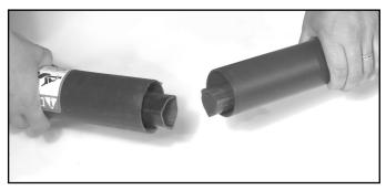
Slide the PTO shield back by using a screwdriver to apply pressure and release the locking collar. (There will be 3 tabs on the locking collar) Once the locking collar is released, slide the PTO shield back.
