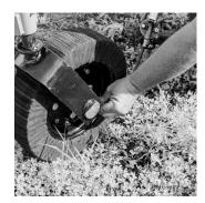
5. Using a 7/8" wrench, remove the fill plug and using a 7mm wrench, remove the drain plug. Both are located on the backside of the gearbox.
