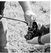
2. Grease the two fittings on each end of the PTO Shield.
