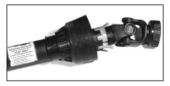
3. Slide universal joint cover up tube toward universal joint. Align grease fitting on shield with white square tabs on collars. This will properly align the position notch and all three (3) tabs.
