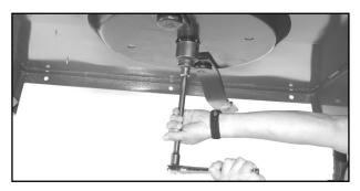
7. To reinstall blade pan, reverse the above steps. Be sure to tighten the castle nut and replace the cotter pin.
