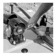
Fill the gearbox with 80W/90 or 85W/140 gear oil until level with the drain plug. (Holds approx. 1 quart)
