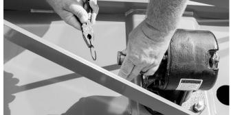
19. Slide the PTO shield back by using a screwdriver to apply pressure and release the locking collar. (There will be 3 tabs on the locking collar) Once the locking collar is released, slide the PTO shield back.
