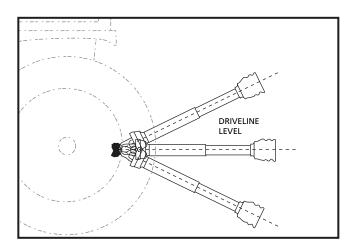
Figure 3 - Check Driveline Maximum Angle
