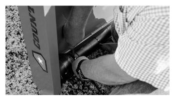
Remove 3/8" - 16 x 2" bolt and nut from the tailwheel holder on the shipping boot, using a 9/16" wrench.
