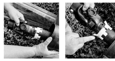
4. If needed, separate white tab collar and slide shield tube back.
