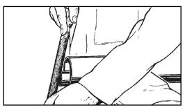
5. Chains must be fitted so as to allow sufficient articulation of the shaft in all working positions.
