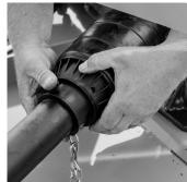
4. Grease the two fittings in the rear tailwheel assembly.
