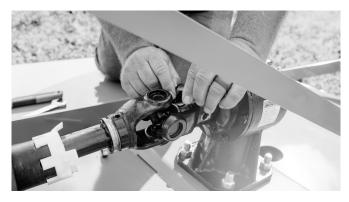
23. Align the shear bolt holes, install, and tighten PTO shaft shear bolt.
