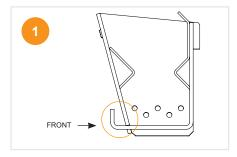
Confirm three baffles inside firebox are secure, placing the side baffles before the center
