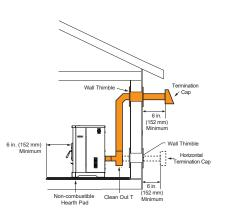
NOTE: In Canada when using a factory-built chimney it must be safety listed, Type UL103 HT (21000F) CLASS "A" or conforming to CAN/ULC-S629M, STANDARD FOR 650°C FACTORY-BUILT CHIMNEYS.
