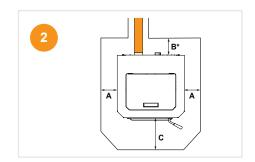
Non-combustible floor protection extending beneath the flue pipe is required with horizontal venting or under the top vent adapter with vertical installation.
