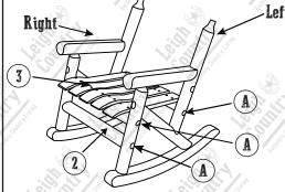
Insert the other arm frame on the other side and secure loosely with nuts and bolts.
