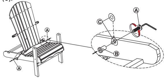
STEP 4 Attach the Right Arm (6) and the Left Arm (5) to the Front Legs (1) with 2 Bolts (A), Washers (B) and Nuts (C). Then attach the Right Arm (6) and the Left Arm (5) to the Back Panel (3) with 2 Bolts (A).
