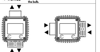
PULSER VERSION The Pulser version is a pulse emitter (reed bulb) which translates the magnetic field variations generated by TURBINE rotation into electric pulses to be sent to an external receiver to be connected. The pulser does not need any independent electric power supply, as it is directly
