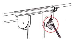
6. Use the provided wood screws to mount each of the lift assemblies (3 screws each) to the ceiling and ensure the distance between the two matches your measurement in step 1.
