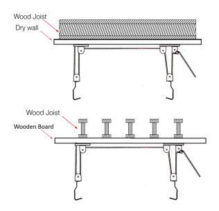
3. Feed rope through the square hole on the back lift assembly. Tie a double knot on rope end as shown.
