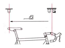
2. Find a suitable location with sufficient wall clearance. Locate a solid wood ceiling joist. Use a screwdriver or a small nail to drill a pilot hole into the ceiling to ensure you've located a joist.
