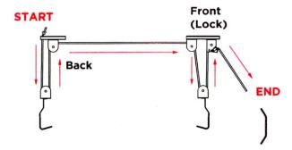
5. Thread the rope down through both parts of the locking mechanism.
