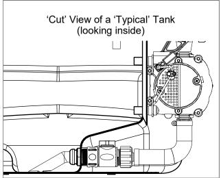
The suction line of your sprayer should contain a 'siphon tube' or intake tube which should be rotated so that it just touches the bottom of the tank surface. (see Detail Views). Reach in and rotate it, as needed, if not already in this position.
