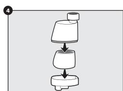
5. Insert the filter housing into the hole on top of the pump.
