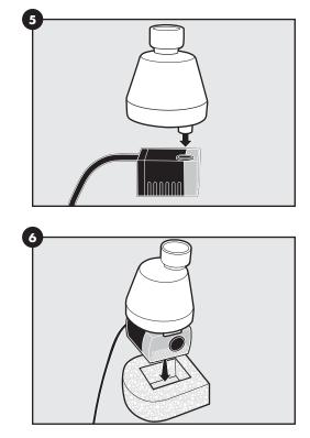
Place the assembled pump and filter housing into the foam filter with the cord running above it.
