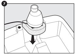
Once the pump is securely in place, feed the cord through the hole on the back of the bowl and out the notch on the bottom of the bowl.
