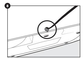
9. Remove the extra slack from the cord and push the rubber seal firmly into the hole.
