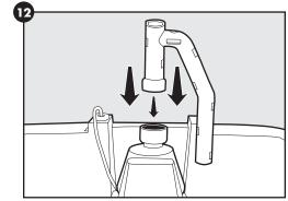
13. Attach the tower by aligning it with the raised notches on the back of the bowl.
