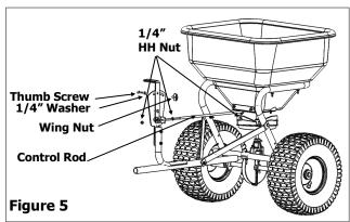
7. To cross-check the proper alignment of the control rod set the Wingnut using Thumb Screw at "2.5" position marked on the Number Pad. Adjust the Adjustable Handle. See Figure 6.
