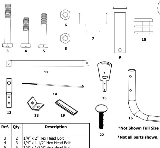
1/4" x 1-3/4" Hex Head Bolt 1/4" Hex Head Nut 6 1 1/4" Wing Nut 12 1/4" Nylock Nut 8 1/2" x 1 3/4" Clevis Pin 2 1" Tube Plug 10 #14 Hitch Pin Clip 11 1 2 Support Brackets 12 13 2 Clevis Plate 1 Upper Rod 14 Number Pad 15 1 16 1 T-Handle Adj. Handle 17 1 Adj. Handle Tab 18 1 Handle Grip 19 1 1/4" x .75" Hex Hd Bolt (Not Shown) 20 21 22 1/4" Washer (Not Shown) 1/4" x 1" Spade Thumb Screw
